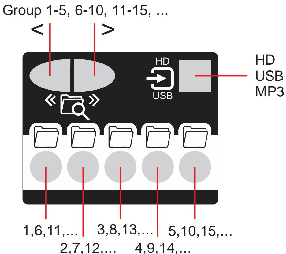
On the top right, the squared button is used for selecting the medium. With this you can select the hard disk, the MP3 player or the USB stick if it is connected. On the top left there are two arrow keys with which you can browse through the groups on the hard disk, MP3 player or USB stick. Each group contains 5 positions. The 5 round buttons represent these positions. Each position is indicated by a number.
