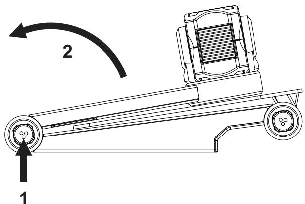
3. Press the large round button in the hinge between the arm and the foot. The button has 3 tactile dots.
