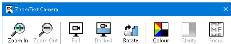
If the Camera toolbar is not in view, press CAPS LOCK + CTRL + C to engage the camera layered key command mode and then press T to bring the toolbar into view.
